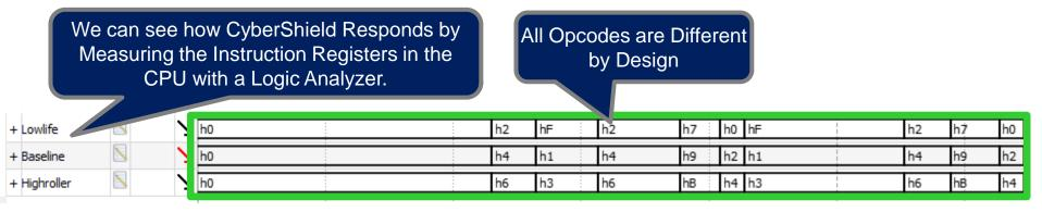
The attack is detected when all three CPUs see the same Opcode. CyberShield Halts Operation and Initiates a Recovery Procedure.
